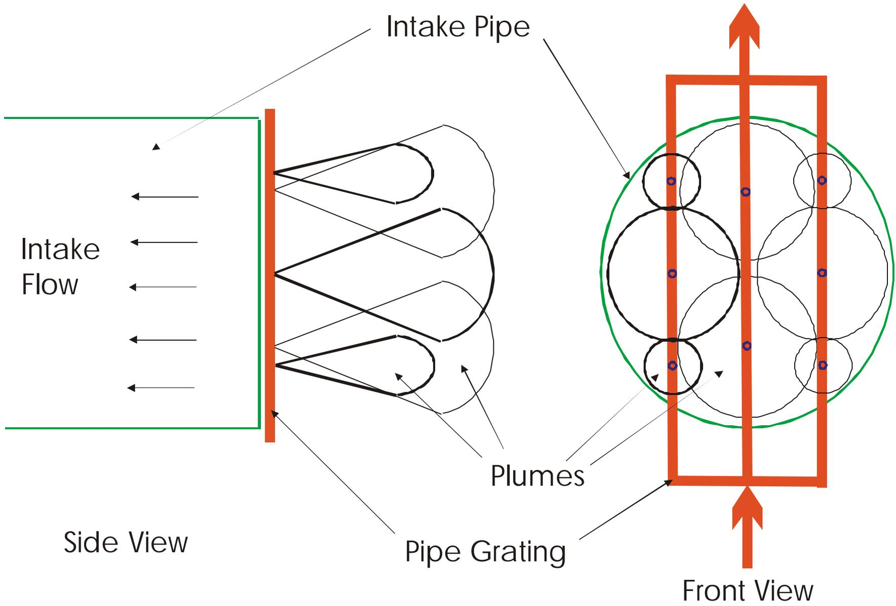
Figure 1: Optimum Jet Dispersion
