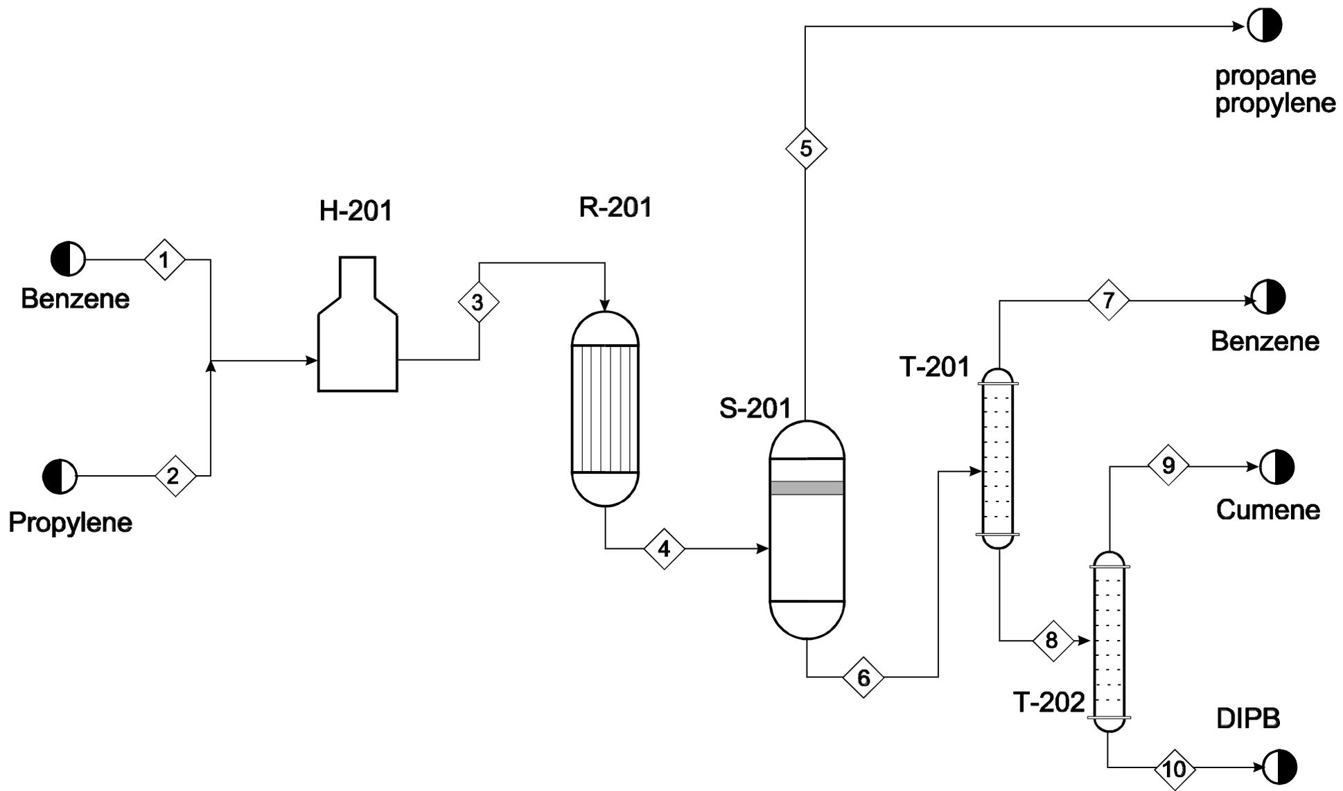
Figure 1: Preliminary Process Flow Diagram for Cumene Production
