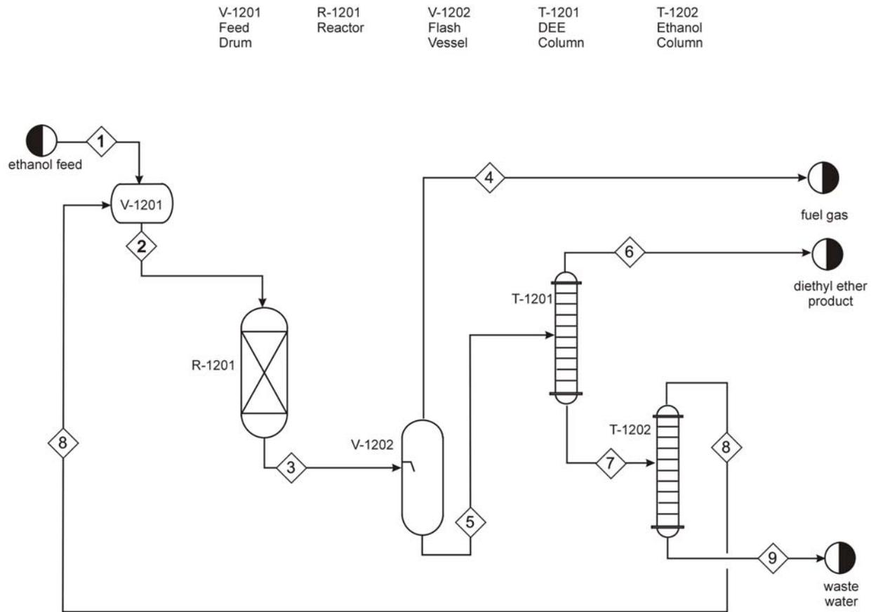
**Figure 1: Unit 1200 Diethyl Ether Process**
