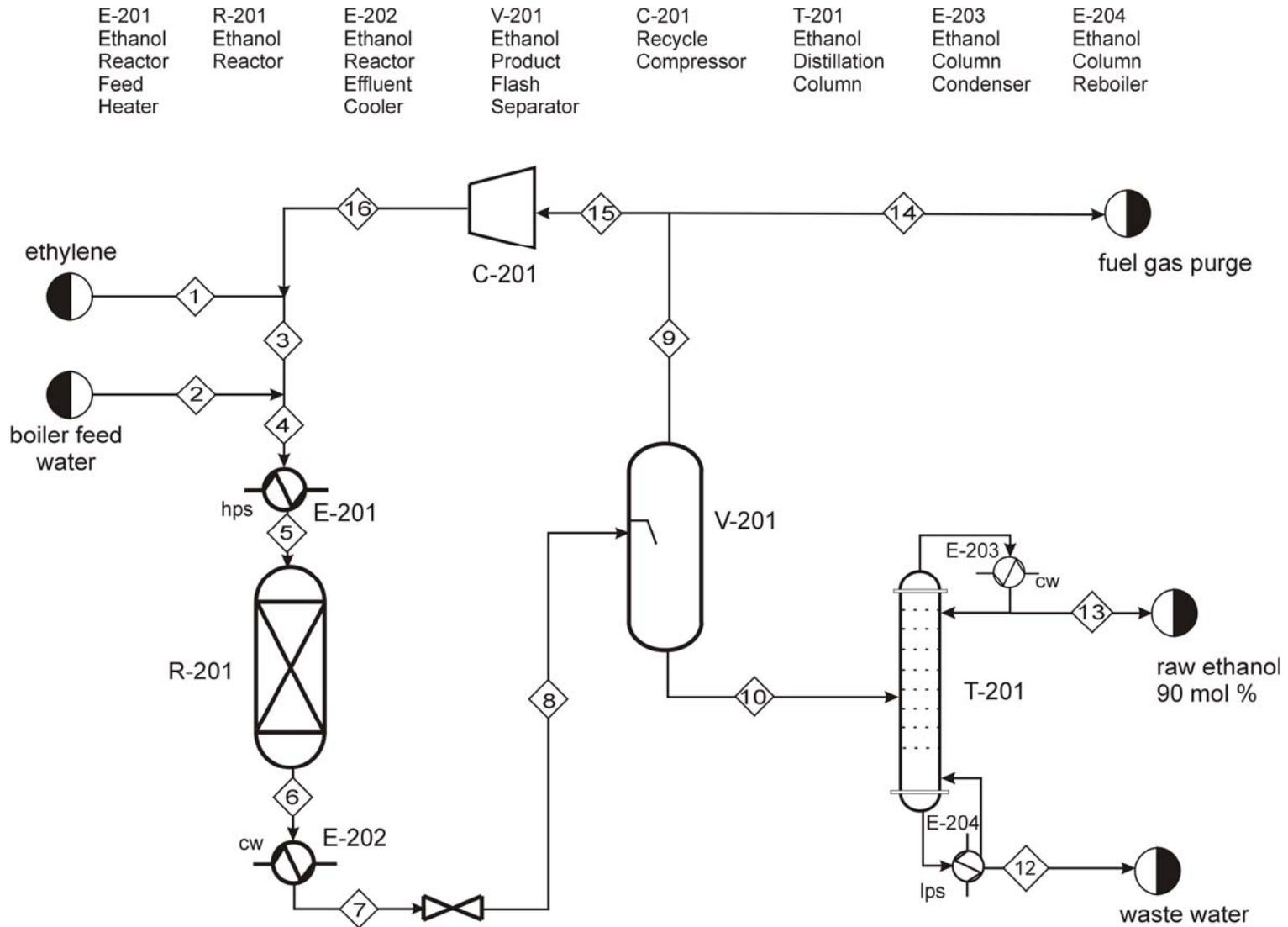
Figure 1: Unit 200 Ethanol Production Process
