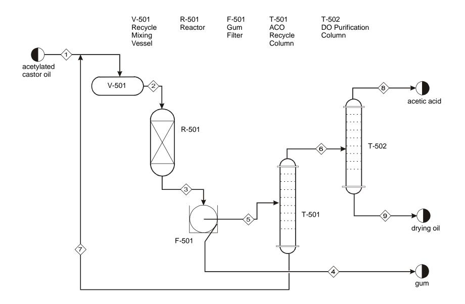
Figure 1: Preliminary Process Flowsheet for Drying Oil Production
